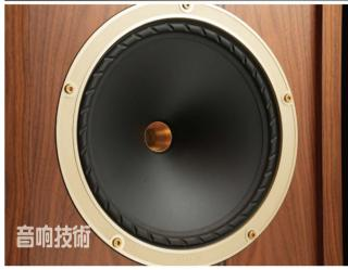
The Vintage Fifteen's tweeter is Fyne Audio's top-tier 75mm titanium dome compression driver, powered by a robust neodymium magnet for smooth high-frequency extension. A gold metal diffuser cylinder connects the tweeter to the mid/ bass driver, ensuring focused high-frequency energy transmission. The crossover is set at 750Hz—lower than typical two-way speakers—meaning the compression driver handles midrange duties, allowing the woofer to focus on dynamics.
